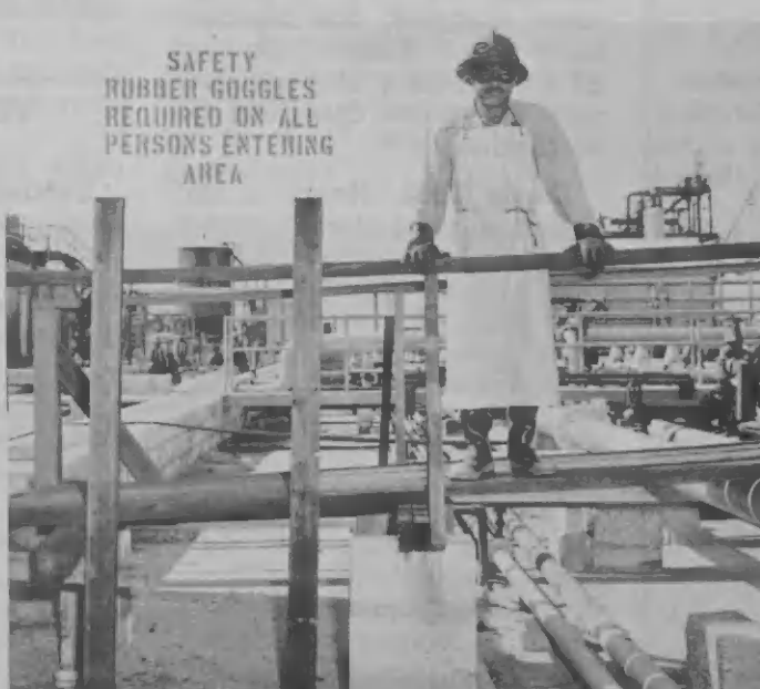
CLEANOUTMEN USE rubber boots and gloves, rubber type goggles and apron against corrosive chemicals. TRAHADOR DI Cleanout ta usa botas y handschoen di rubber, bril y lantera contra quimico corosivo.
